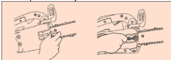
Fig 30: Adjusting the tension so the straps and cutters solidly contact the bar rail
